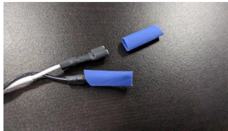
3) Finish the unused Purple/Black & White/Black wire ends with tape or heat shrink.
