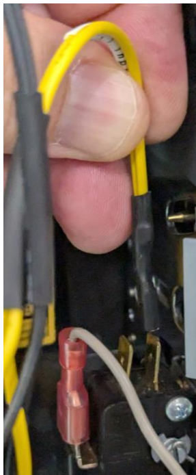
11) Connect the Yellow Coin In from the AmusementConnect harness to the coin mechanism.
