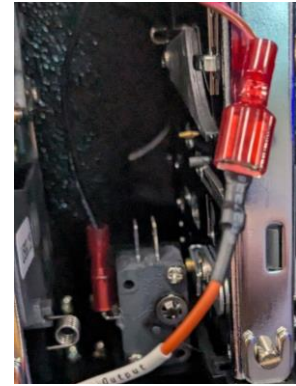
6) Connect the Orange Coin Pulse Output line from the AmusementConnect harness to the coin line disconnected in the previous slide.
